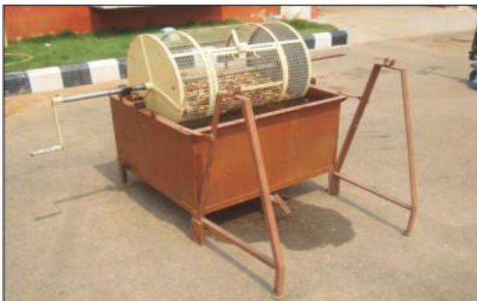
Figure 6: Square-mesh drum ginger peeler
